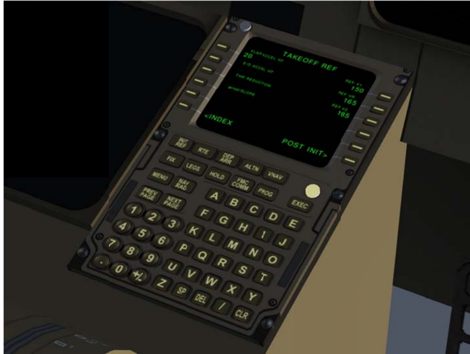
Figure 7 Boeing 747-400 CDU ( http://wiki.flightgear.org/File:747-400_CDU.png )
