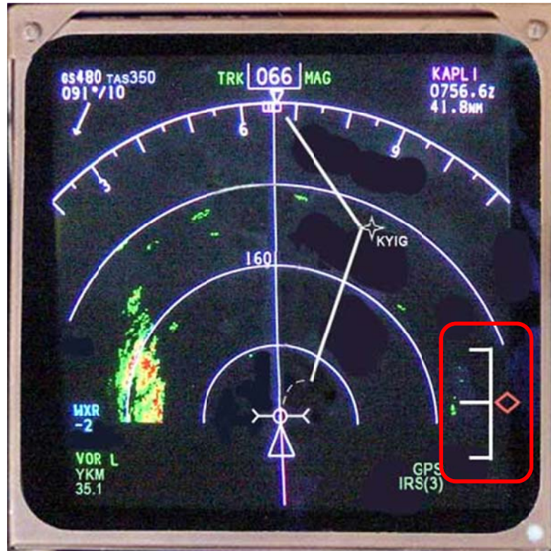
Figure 6 Boeing 747-400 ND with vertical deviation indicator highlighted in red box (photo retrieved and adapted from http://www.meriweather.com/747/fd-747.html )
